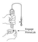
2. To prep syringe, simply aspirate up to 20ml of contrast solution or fluid to be dispensed into the inflation syringe by pulling back on the plunger handle.
