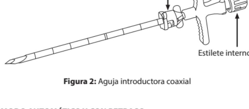
**Figura 2:** Aguja introductora coaxial
