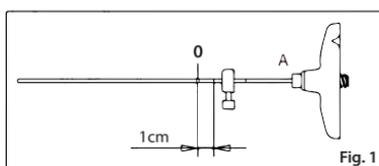
Fill a syringe with cement of choice (not supplied, using manufacturer's directions to achieve desired viscosity), attach to the luer end of Filler (A), and fill with cement.
