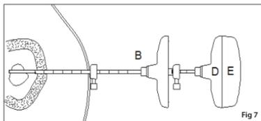
Then rotate Biopsy Needle and Handle (D+E) counterclockwise and remove. Remove the Handle (E) from the Biopsy Needle (D); insert the Ejector Pin (F) through the Biopsy Needle (D) from the luer end and eject the sample.
