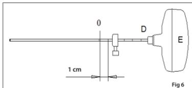
**Note:** The selected centimeter marker (see Fig. 6) will represent the Biopsy Needle (D) protrusion beyond Cutting Cannula (B).
