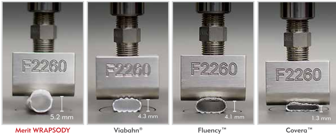
Merit WRAPSODY versus 10 mm leading covered stent, each compressed by 1.8 N.
