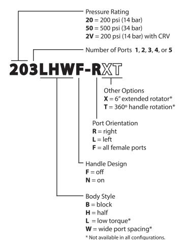
Merit's DeVos manifolds are a standard manifold with a check relief valve as the end port. The DeVos manifolds are available with: 2 or 3 port standard port spacing and 4 port wide
