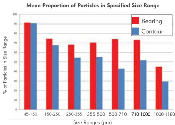
For all seven size ranges, on average, **Bearing nsPVA** had **33%** more particles in the specified size ranges than Contour.
